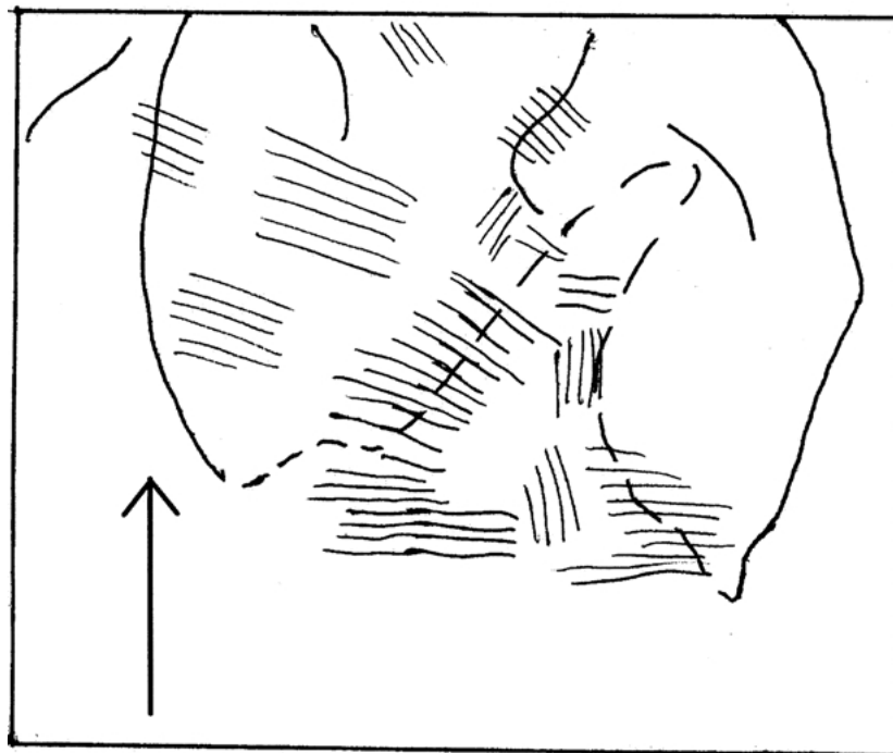
(b) Dotted line is the SCC-FFS interface. Parallel lines are pearlite colony orientations. Large arrow is crack growth direction.
