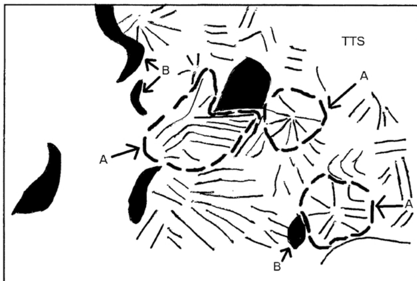
(b) Schematic view showing TTS. A: Flat region (bounded by dashed line) B: Chasm or secondary crack
